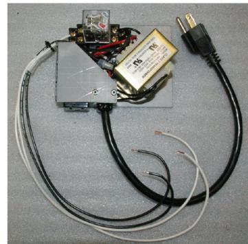
Connect the two white wires to a milli volt valve, a SIT electronic Ignition system or a post purge control system for a power vent module instead of the wall switch.
