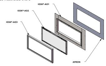
Back frame the unit with the metal header supplied by Montigo above the unit and either combustible or non-combustible framing to the sides and bottom maintaining clearances as shown and ensuring the galvanized apron can be attached to the framing.
