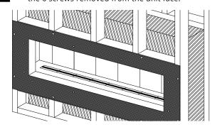
Install the silicon gasket material (supplied by Montigo) in one continuous strip with the joint at the bottom
