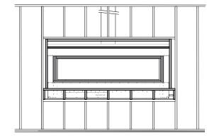
CLEARANCE TO COMBUSTIBLES: 6" Top, 3" each side, 3" bottom from the protruding window box.
