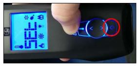
5. Keeping pressed the Power On/Off button, press the Up button to set the icon. And remove the symbol from the screen.
