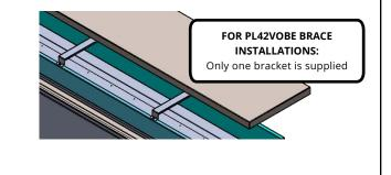
Fasten Electrical Box to PART №14 Electrical BoxBracket with (2) ¼-20 x 3/8" long Pan Head Screws
