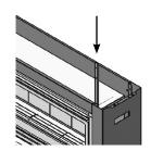
**11**Fasten PART №15 Braces to rear panel assembly and<br/>Panel Top front with (2) ¼-20 x ½" long Pan Head<br/>Screws.
