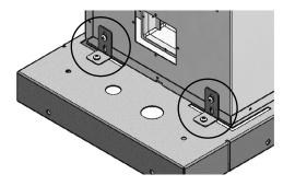
Level out the unit with the attached Hex bolts **PART** №HW2302 and Nuts **PART №HW2145** on the bottom of the pedestal.
