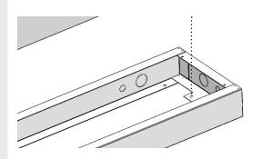
Knock out gas and electrical access ports in base if necessary, inset bushing PART № HW6006 and electrical clamp connector PART № EC1220. Run gas and electrical lines through the ports
