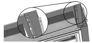
Slide PART №7 Brace over the front and side panel and secure with (4) ¼-20 x ½" long Pan Head Screws as shown. Repeat on other side with PART №8 Brace and (4) screws.
