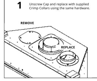
Secure Heat Distribution kit to Framing at Desired Height and use supplied crimp collars to secure ducting
