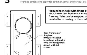
Plenum has 6 tabs with finger bends to attach to either horizontal or vertical framing. Tabs can be snapped off if not needed for screwing to the stud.
