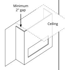
**Figure 19.e** Open top chase venting on top of enclosure
