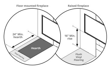
The minimum depth of the hearth is 24" if the fireplace base is flush with the floor (ie; not raised, and not recessed into the floor)
