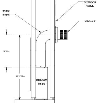
Figure 4.bb Minimum Horizontal vent run (Flex)
