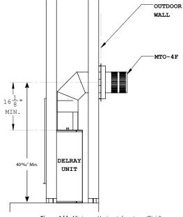
Figure 4.bb Minimum Horizontal vent run (Rigid)
