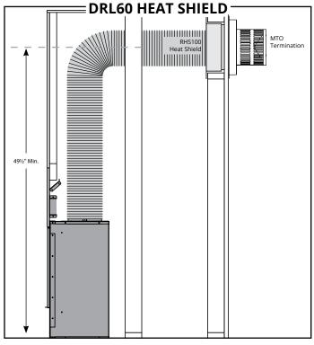
Figure 15.b RHS100 Installation. (Minimum requirements).
