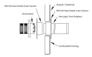
**Figure 15.c** RHS100 Installation. (Install by sliding Outer Section over vent pipe where it passes through the combustible construction.
