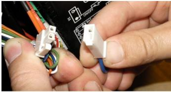
Figure 19.b Locate Jumper cable
