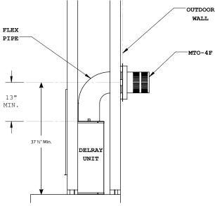
Figure 4.bb Minimum Horizontal vent run (Flex)
