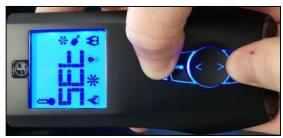
4. Keeping pressed the Power On/Off button and pressing the O button, navigate to the Transmission icon. This is in Clr state.
