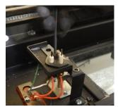
Figure 13.f Insert propane orifice, reassemble burner
