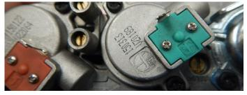
Figure 13.h Adjust pressure ports
