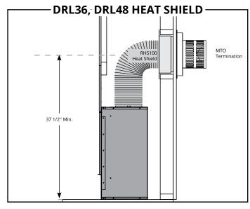
Figure 15.b RHS100 Installation. (Minimum requirements).
