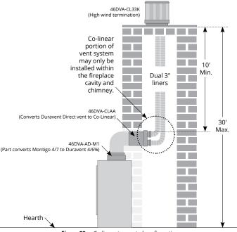
Figure 99.a Co-linear top vented configuration.
