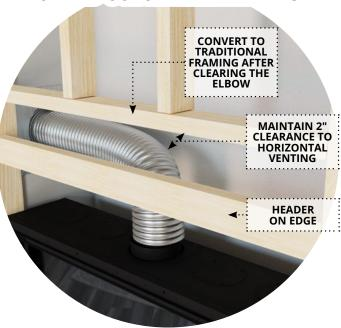
The use of flex venting in the scenario shown above makes the installation easier as it allows for a lower combustible header height AND accommodates the bend the vent has to take due to the shallow framing depth.
