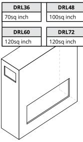
**Figure 19.b** Side chase venting on both sides of enclosure
