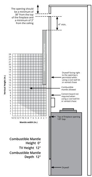
Figure 19. Combustible mantles and facings. (Not to scale)
