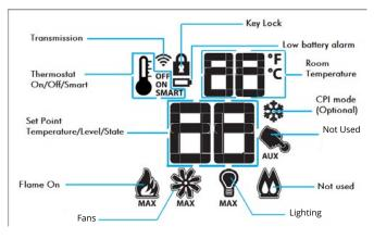
Figure 29.c Remote Control LCD Display
