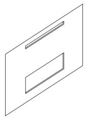
**Figure 19.d** Front chase venting on front of enclosure
