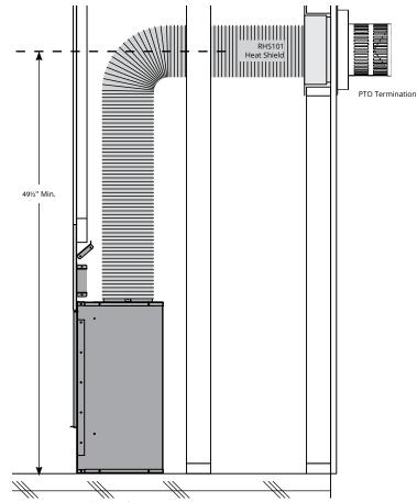
Figure 15.b RHS101 Installation. (Minimum requirements).
