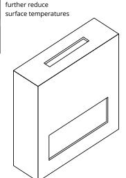
**Figure 19.c** Top chase venting on top of enclosure
