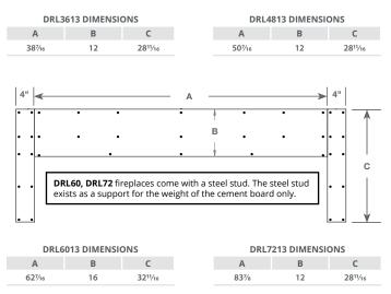
Figure 28. Supplied non-combustible cement board dimensions
