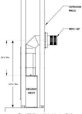
Figure 4.bb Minimum Horizontal vent run (Rigid)
