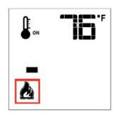
Figure 27.g Flame Off and Flame Level 1.
