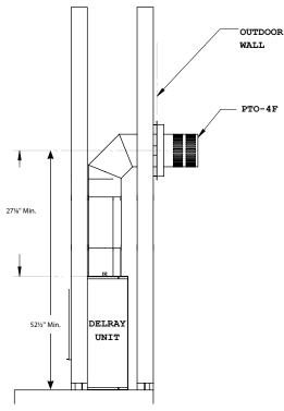
Figure 4.bb Minimum Horizontal vent run (Rigid)
