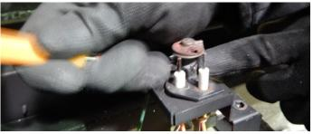
Figure 13.d Removing the spring clip
