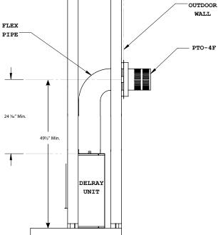
Figure 4.bb Minimum Horizontal vent run (Flex)
