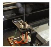
Figure 13.f Insert propane orifice, reassemble burner
