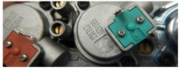
Figure 13.h Adjust pressure ports
