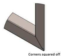
The Trim slides on the inside of the flush frame of the opening. Push in until the trim is flush with the facing material.
