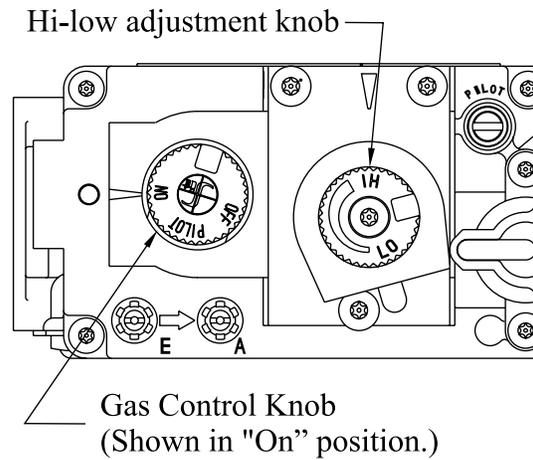
Figure 9. 'Hi-Lo' Adjustment on the M38DV-PFC gas valve.
