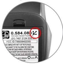
The above transmitter will not sync with the IFC control module RGC3095 which can be identified by the white stencil on top
