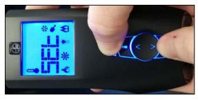
Keeping pressed the Power On/Off button and pressing the O button, navigate to the Transmission icon. This is in Clr state.
