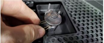
Figure 13.d Removing the spring clip
