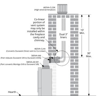
Figure 99.a Co-linear top vented configuration
