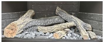
Step 7: Log  ${\bf H}$  is placed in the center of the firebox with the thin end resting on log  ${\bf B}$
