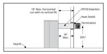
Figure 9.b Straight run, Rear Vented, wall mounted termination.
