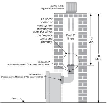
Figure 99.b Co-linear rear vented configuration
