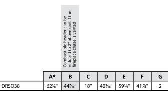
\* This is the minimum dimension, number can be greater than listed. Some venting configurations that require more vertical rise will require a larger enclosure to provide minimum vertical clearance between vent pipes and combustibles
