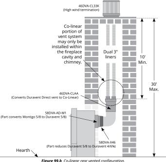
Figure 99.b Co-linear rear vented configuration.
