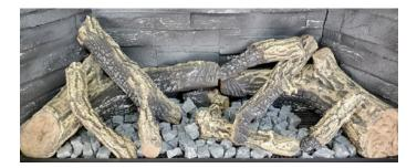
Only cover the burner with one layer of coals. Arrange the ember chips on top of the burner tray. DO NOT cover the pilot with logs.
