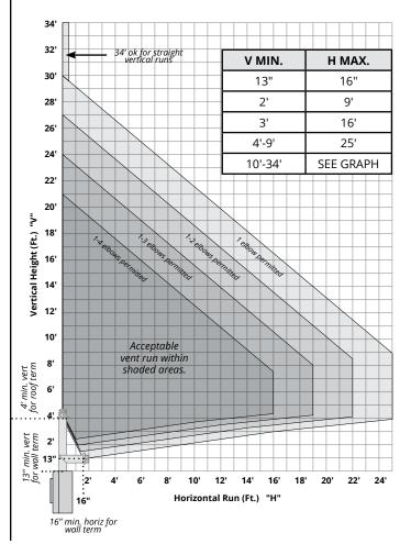
\*4" vertical minimum is based on the vent center of an elbow mounted directly on the top of the unit.
