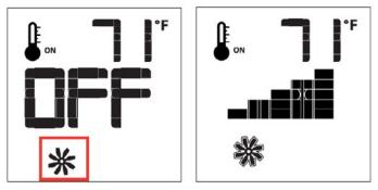
Figure 27.m Fan Speed Control
