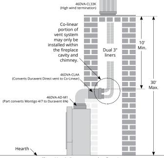
Figure 99.a Co-linear top vented configuration.
