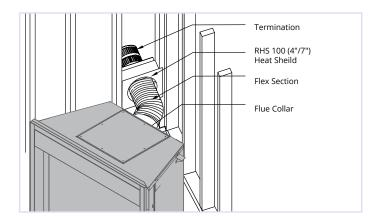
**NOTE:** The MVK05 / MVK05F kit is available for top vent corner FLEX application (NG only). The Kit includes a heat shield, flex pipe, and a termination with or without a mounting frame.
