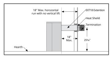
Figure 9.b Straight run, Rear Vented, wall mounted termination.
