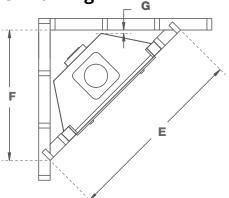
Figure 3.b Framing dimensions (Straight wall & Corner Installation).
