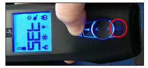
5. Keeping pressed the Power On/Off button, press the Up button to set the icon. And remove the symbol from the screen.
