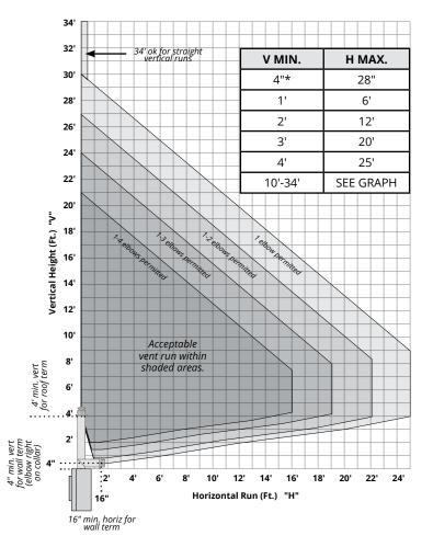
\*4" vertical minimum is based on the vent center of an elbow mounted directly on the top of the unit.
