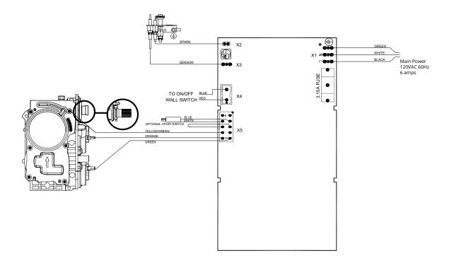
Figure 15. Wiring diagram for DRSQ\*\*\*I with SIT Proflame Electronic Ignition
