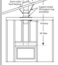
Figure 6. Top vent, roof mounted termination with no offset in vent run.
