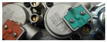
Figure 13.h Adjust pressure ports
