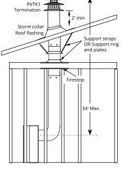
Figure 6.d Side vent, Roof mounted venting (1 = 90° bend).
