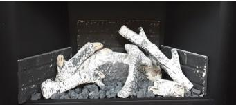
Only cover the burner with one layer of coals. Arrange the ember chips on top of the burner tray. DO NOT cover the pilot with logs.
