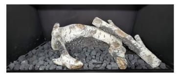
**Step 5:** Place log **C** at the left corner of the firebox, with the charred side facing the middle of the media tray
