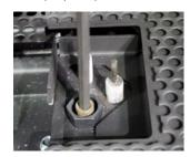
Figure 13.e Removing the pilot hood, orifice
