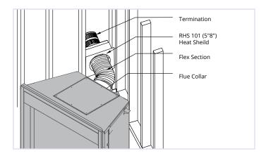
**NOTE:** The PVK05 / PVK05F kit is available for top vent corner FLEX application (NG only). The Kit includes a heat shield, flex pipe, and a termination with or without a mounting frame.
