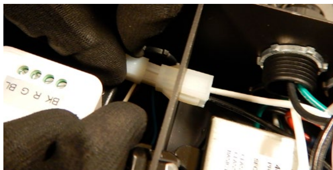
Figure 34 Connecting the LED receiver
