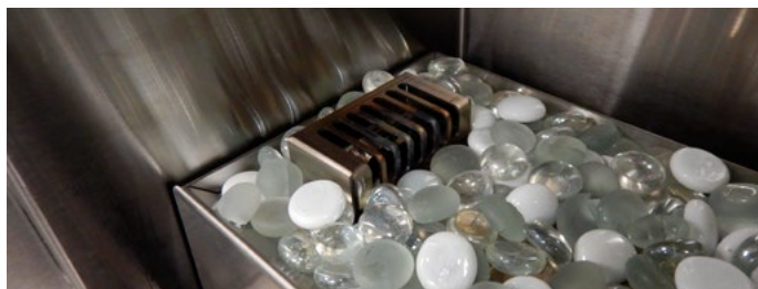
Figure 66 DO NOT place ANY firestones on top of the pilot cover).
