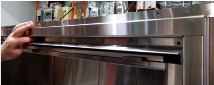
Figure 56 Removing the left side screw
