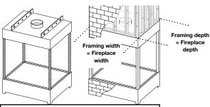
Any framing on the top of the fireplace must be noncombustible, and externally supported. Framing can be in contact with the hood, but must not use the fireplace hood to support the framing. After framing is complete, finishing materials can be extended down along the face of the unit. Do not obstruct the glass opening with finishing materials.
