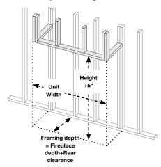
† There are no restrictions on mantel clearance providing they do not project beyond the facing material edge, and the weight of the mantel is fully supported by the framing. Combustible mantels must not be in direct contact with fireplace. ie. A mantel must have a noncombustible underlay between the fireplace and mantel.
