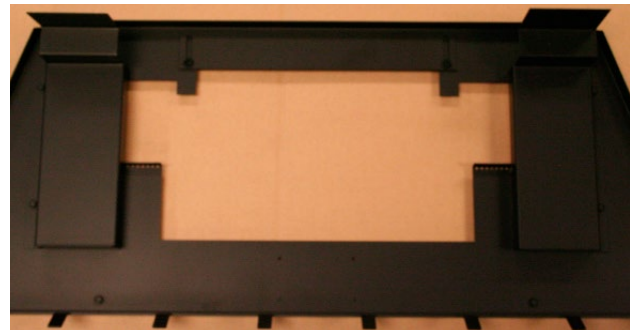
Figure 8b. Air Baffle in Open position
