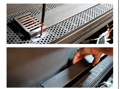
The ten (10) screws that retain the media tray can now 2 be removed. Remove the two media tray(s) as shown below.
