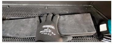
2 The screws that retain the media tray can now be removed. Remove the media tray as shown below.
