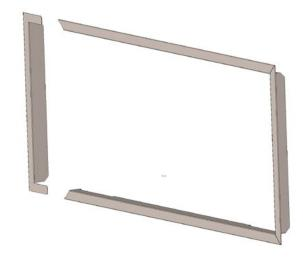
Ensure the all 4 corners of the trim kit are squared off. Before installation orient the trim so the notched section is on the bottom.
