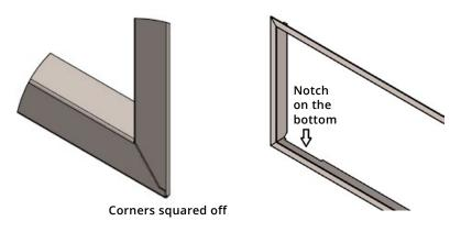
The Trim slides on the inside of the flush frame of the opening. Push in until the trim is flush with the facing material.
