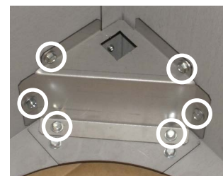
Figure 3.e Unscrewing control cable cover
