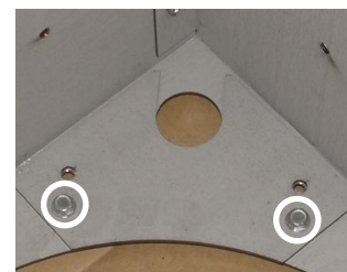
Figure 3.f Removing strain relief plate.
