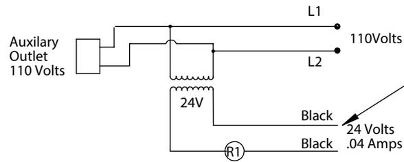
Connect the two black wires to a Lutron/ wireless remote control or any other switch. The two black wire will control a 24 Volt relay. Specifications: 24 Volts AC current is 4 milli Amps
