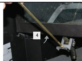
Figure 6.g Lift the door up and out of the fireplace frame
