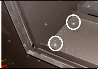
Figure 4.b Removing screws that secure media tray
