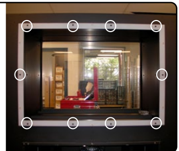
Figure 6.g Removing screws that secure screen.
