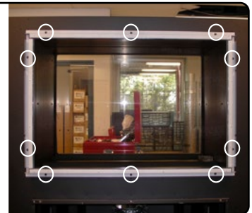
Figure 6.f Removing screws that secure screen.
