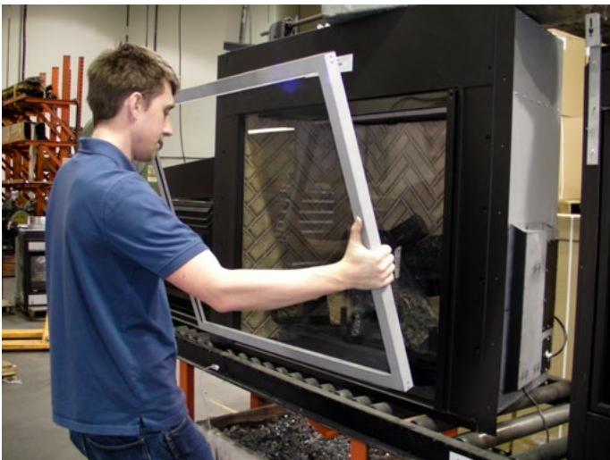
Figure 16b. Lift screen off retainer slides.
