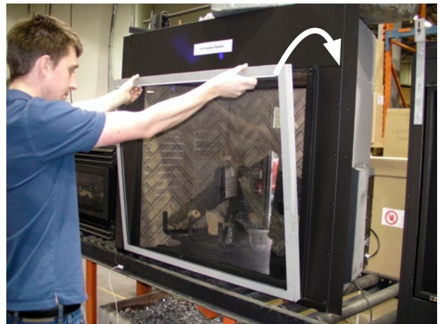
Figure 17d. Pushing screen into place.
