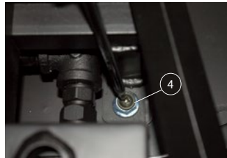
Figure 20b. (RH Base mounting machine screw).
