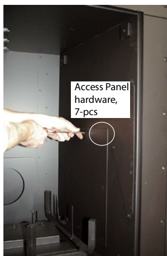
Figure 26. (Removing the panel hardware).
