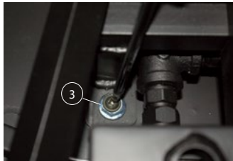
Figure 20a. (LH Base mounting machine screw).
