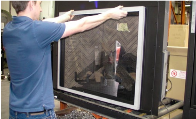
Figure 16. Lifting top edge of screen.
