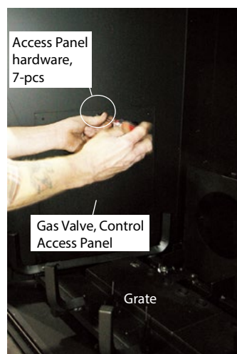
Figure 28. (Removing the panel hardware).
