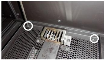
Figure 107. Pilot end of burner tray.
