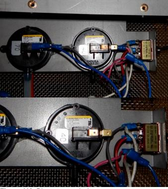
Figure 113. Disconnect red wire.
