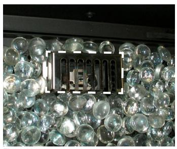
Figure 61. Do not place any media on top of the pilot shield.
