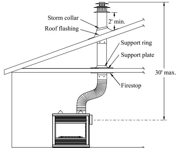
Figure 17. Vertical venting using 1 offset (1 offset= two 90° bends).
