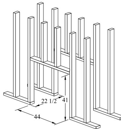
Figure 2a. Framing dimensions for the rough opening.
