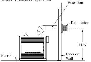
Figure 13. Short Horizontal Installation.
