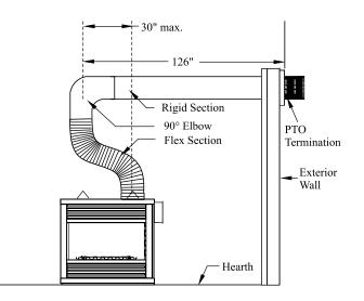
Figure 14b. Retracted Installation.
