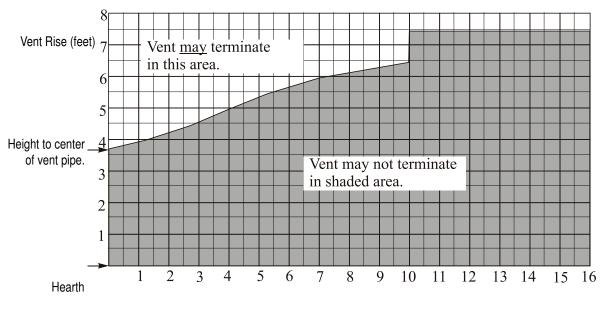
Figure 12. Rear Vent Venting Graph.
