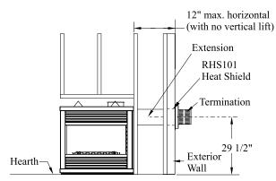
Figure 7. Short horizontal installation.
