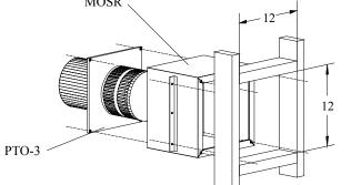
Figure 4c. Installing a PT0-3 termination with the MOSR frame.
