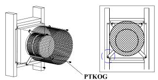
Figure 4d. Installing the heat guard.
