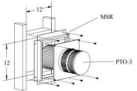
Figure 4b. Installing a PT0-3 termination with the MSR frame.
