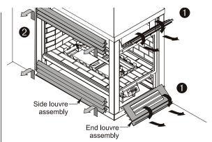
Figure 22a. Removing the louvre assemblies.
