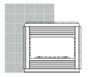
Figure 20c. When using a tile surround, do not tile over the outside
