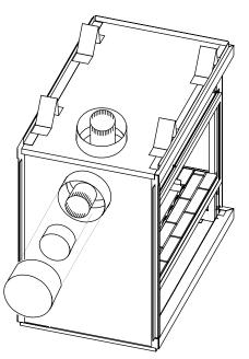
Figure 5a. Installing the flue cover.
