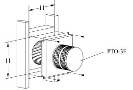
Figure 4a. Installing a PT0-3F termination.
