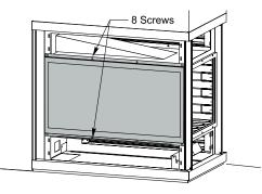
Figure 22c. Removing the door.
