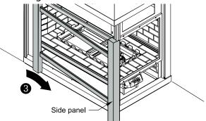
Figure 22b. Removing the side panel.
