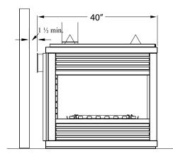
Figure 2b. Flue Cover clearances to combustibles when installing the unit in a top vent configuration.
