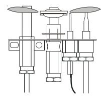
Figure 26. Pilot Burner
