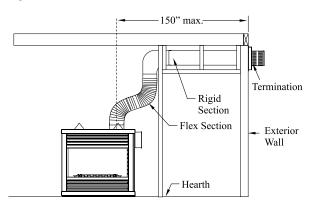
Figure 14a. Extended installation.
