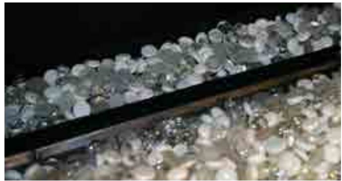
Figure 25. Completed firestone installation. Second Gen burner shown.
