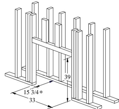
Figure 2. Framing dimensions.
